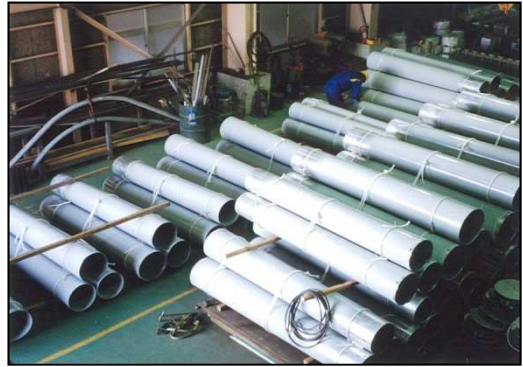
Lightweight steel poles (panzer masts)
